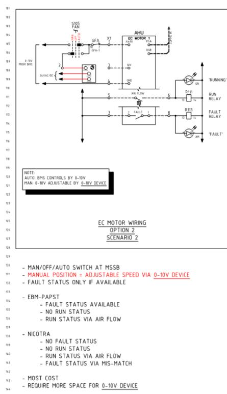
Option 2 – Scenario 2 – manual position via 0-10V using independent 0-10v device, refer to Belimo examples below
