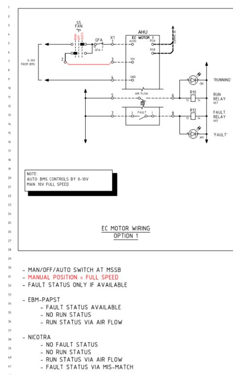
Option 1 – Fixed Speed in Manual setting where variable fan speed is not required
