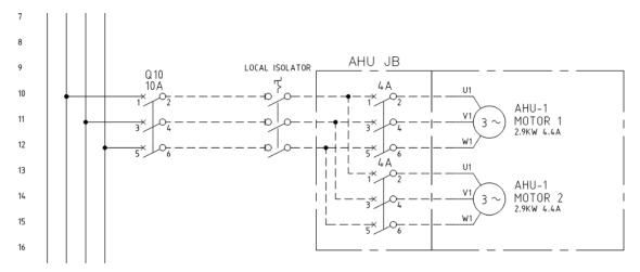
Irrespective of the number of fans per unit, consideration must be made for CTs on the power supply to each fan to aid with run and fault monitoring, interfaced to MSSB and BMS, particularly for manufacturers who do not provide HLI run/fault information and more prevalent on multi fan units.
