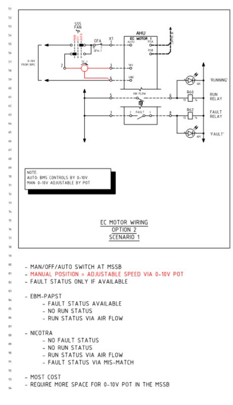
Option 2 – Scenario 1 – manual position via 0-10V POT - 10v from EC motor (for most installations)
