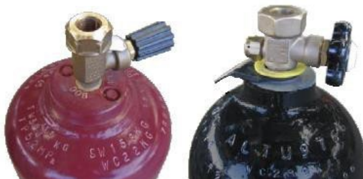
Figure 13 Oxygen and acetylene cylinder valves
