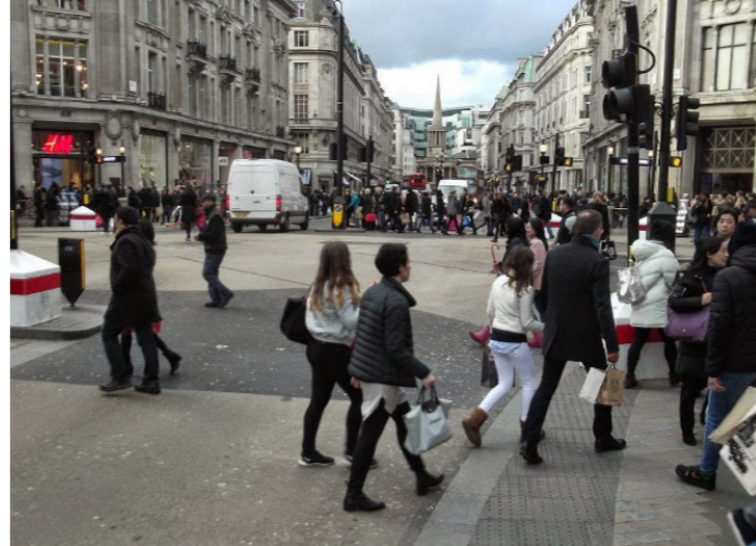
Figure 10: Oxford Circus, London (right) – Blister paving provided full length along pedestrian crossing.
