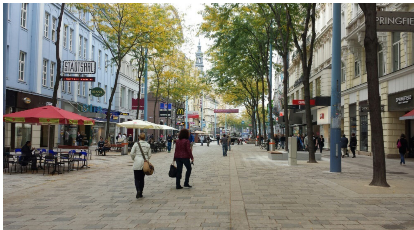
Figure 6: Mariahilfer Straße, Vienna – A continuous and flat paving type solidifies the area as a shared zone, giving no priority to vehicular traffic, and encourages pedestrians to inhabit the entire space.
