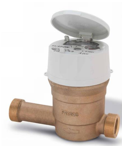
Figure 6D – TD 8 Rotary Piston Volumetric type water meter
