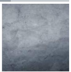
Element: larger terraces Indicative Material: in situ concrete, smooth, washed finished
