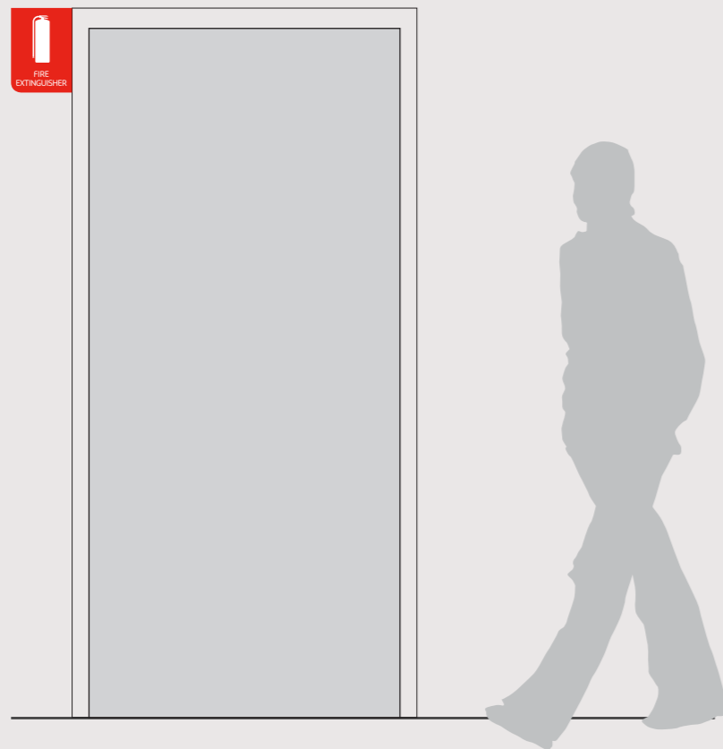
Installation Guide: A - Left of door Scale 1:20
